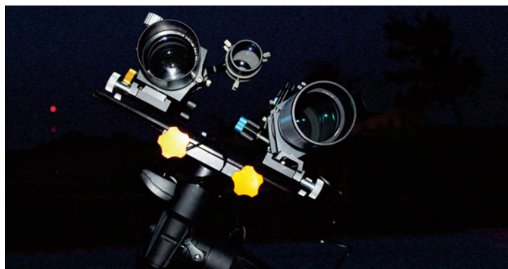
Image 14 - The author tested the Askar 71F side by side with a Stellarvue SV70T. These two scopes are closer in focal length (420mm and 490mm) than his two Askar models.
