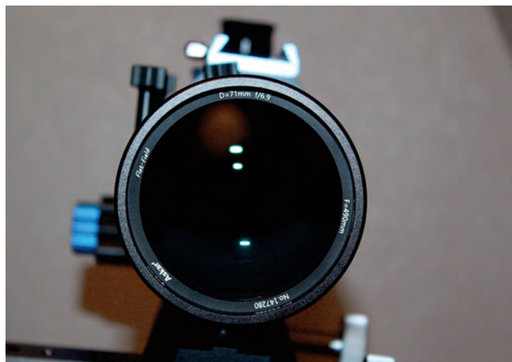
Image 3 - The objective is 71mm in diameter and has a focal ratio of 6.9 providing a 490mm focal length.
