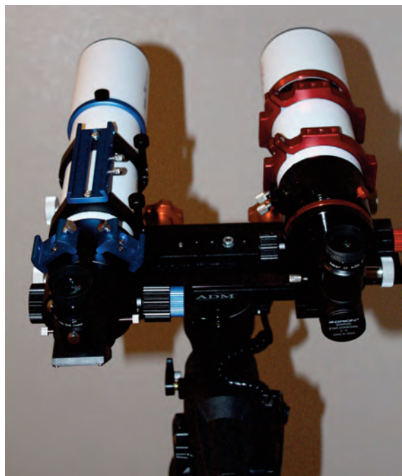
Image 9 - There are three places to attached accessories atop the 71f (left) than on the FRA400 (right). The FRA400 did come with a handle attached to the top of the tube rings, which I had removed to lighten the load.
