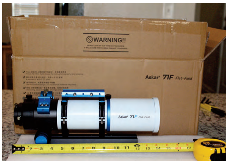
Image 4 - With the dew shield fully retracted, the telescope is 14.67 inches (372.5 mm) long.
