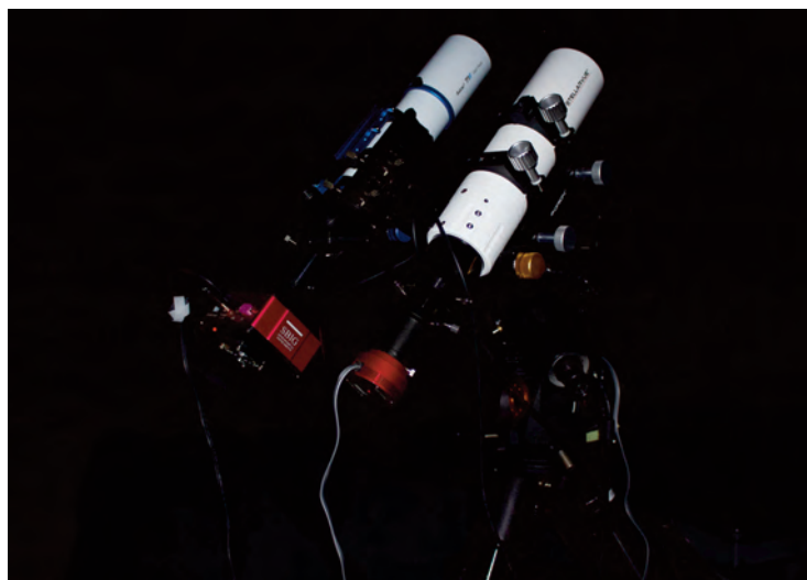
Image 18 - The author took long exposure CCD images through the Askar 71F using an SBIG STF-8300C camera guiding through the Stellarvue refractor.
