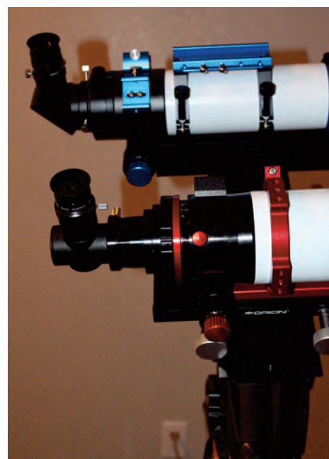
Image 8 - Both Askar telescopes have identical (except for the diameter) and smooth operating two-speed rack-and-pinion focusers.
