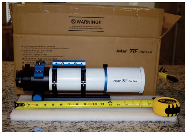
Image 5 - With the dew shield fully extended the telescope is slightly less than 17 inches (431mm) long.
