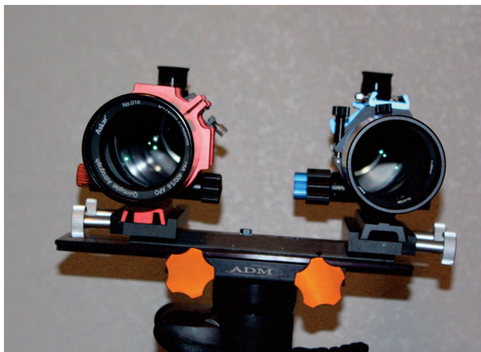
Image 7 - From this view it can be seen that the objective lenses are indistinguishable in diameter. The 71F (right) was made lighter by using a smaller diameter tube and thinner tube rings.
