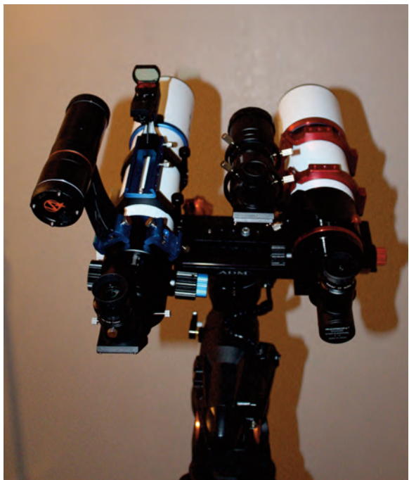
Image 10 - This view shows a 9x50mm right angle finder scope attached the FRA400. There is a red dot finder and a Celestron StarSense auto-guider attached to the 71F.
