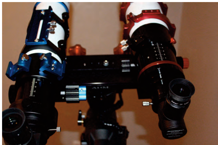
Image 11 - The draw tubes for both telescopes (fully extended here) have graduations that allow recording of focus positions for different eyepieces or cameras. The 71F has a 5cm draw tube while the FRA400 has a 5.5cm drawtube.
